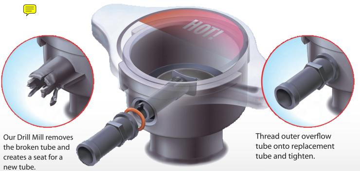
Insert the flanged inner overflow tube and place the O-ring over it.
